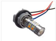
Base for BAY15D bulbs, with wires for connection. The gasket on the lamp secures a waterproof joint in a 26mm hole. There is 120mm cables in the end.
