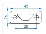
Alu profile in series 40, with 16mm height and one 8mm slot. Can be used for lids and other purposes, that only require one track.
