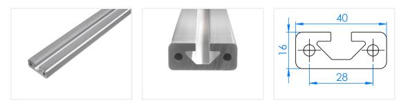
Alu profile in series 40, with 16mm height and one 8mm slot. Can be used for lids and other purposes, that only require one track.
