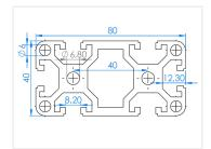
Extra strong double-width series 40 profile, typically called 4080, that eg. can be used as a basis frame in a larger constructon. There are 2 tracks on both sides, and 2 in the ends, with a total of 6 tracks, 8mm. There are also 6 holes that you can cut a thread in.
