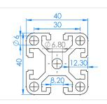
Standard construction profiles in 4040, with basis dimensions 40 x 40mm and a 8mm slot. The profiles are an extra thick model, solid core and round holes.
