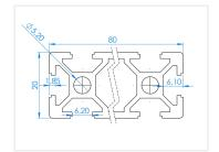
Extra wide series 20 profile, with the dimensions 20 x 80mm and 4 slots / tracks, with 6mm width. The wide profile with the many tracks makes it an advantage to use it as a table in a CNC or similar.
