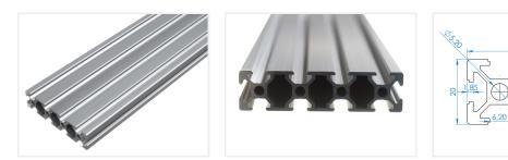
Extra wide series 20 profile, with the dimensions 20 x 80mm and 4 slots / tracks, with 6mm width. The wide profile with the many tracks makes it an advantage to use it as a table in a CNC or similar.
