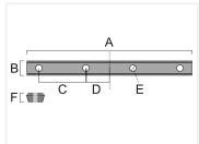
Long joint to make a straight joint of two profiles, end to end. 4 pinol screws ensures it can be fastened securely.
