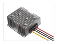
Simple waterproof voltage regulator, that can be used to drive the input voltage from 20-80V down to 12V. The compact aluminium housing works as heatsink, with large cooling fins.
