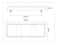
Nice flat LED combination lamp with rear light, indicator and brakelight, and also either reverse light or fog-light. The built-in voltage regulator allows you to connect it to both 12V and 24V. ADR/ECE approved for legal road use.
