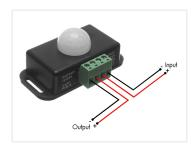
Compact PIR motion sensor with screwterminals on the input and output. The sensor can be used for both 12V and 24V. When the sensor is activated, it will turn off after the set up delay, that can be from 1 to 10 minutes.
