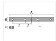
A strong aluminium-bar that fits in to series 40, 8mm slots. 4 large bolts tightens the two profiles securely together.
