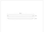
A red strip-lamp that is ECE-approved as a tail light and a brake light. The strip-lamp can be recessed on a surface (cut out 203x19) or you can mount it using a mounting bracket.
