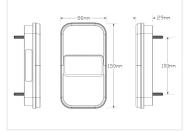
LED lamp with a tail, a brake, and an indicator light. 8 bright LEDs. With and without license plate light. ECE-approved and a 5-year warranty.
