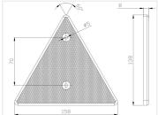
Set with 2 styks ECE-approved triangle reflectors, which are legally required on trailers and semi-trailers. 158 mm on all sides, so it has a height of 138mm.
