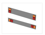
A wide tail light with a tail, a brake and an indicator lamp for 12V and 24V with measurements of only  $8 \times 15$ cm. There is also a built-in reflector. It is available with a 40cm cable or a 10 metres cable.
