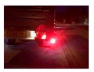
Nice and simple LED stalker lamp in a short flexible rubber base, intended for marking with red and white position light and models with a built-in yellow sidemarking light.
