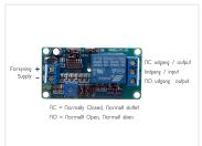
A smart relay with an adjustable on or off function. The delay can be adjusted from 0.1 second to 1 hour. The relay has one input and an output that is normally connected (NC) and another output that is normally open (NO).
