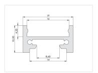
An anodized alu u-profile for LED stripes. A simple, flat and nice profile that can be mounted with hidden clips.
