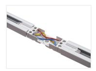
A joint for two tracks with inside screw-terminals for connecting the profiles to 230V. The two ends are pre-connected with cables and so this part can also be used as a simple joint.
