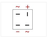
Smart rectifier-bridge that transforms AC to DC. It can be used for LED lighting, where the source is AC.
