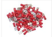
Male lugs with the dimensions  $6.3 \times 0.8 \, \text{mm}$  in red size for  $0.25 - 1.5 \, \text{mm}^2$  wires. Crimped in a matching crimping-tool.
