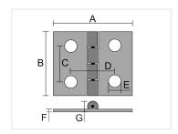
Plastic and aluminum hinges, that can be used for doors and lids. The hinge is fastened with M6 bolts.
