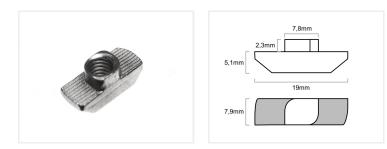
Nut that fits in to series-40 profiles, where after you can put in a bolt. This nut turns itself in to position when tightened.
