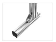
A bracket in aluminium for joining two series 20 profiles in 90 degrees. There are knobs under the brackets to keep them in the slot while tightened. The knobs can also easily be ground down, if you need to mount the brackets transversal.
