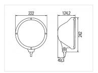
A large auxiliary lamp for mounting on cars and trucks. The large size, but low weight make the lamp useful on larger vehicles. It is made from stainless materiels. The large reflector and the clear front-glass give a great light at long distances.
