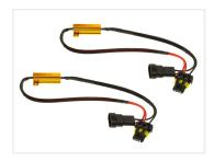
A resistor with 9006 / HB4 plug. Used for LED conversions, where it is put in between the 9006 / HB4 bulb and the car $^{\prime}$  9006 / HB4 plug.
