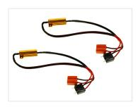
A resistor with a H7 plug. Used for LED conversions, where it is put in between the H bulb and the car' H7 plug.
