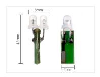
2 very strong 3 mm diodes on the print that fits in 1,2W holders in a heater and contacts that require much light to the sides.
