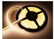
The splashproof LED Tape SMD can be shortened or extended further, so it fits for your project. The stripe is 8/10 mm wide and is built up in small modules of 5 cm or 10 cm, where there are 3-6 heavy SMD diodes in a circuit ready for 12Vdc. There are clear markers where the stripe can be cut, as well as solder-islands, where you can solder wire on or extend with more SMD-tape. On the back is a 3 m powerful tape, which makes that LED SMD tape to stay attached to his seat without screws.
