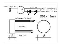
Round LED driver that supplies 350mA constant current. It can handle up to 35V, and can drive up to 9 high power LEDs.
