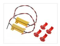
When switching the fog/tail lights with LED styling lamps or the diode bulbs, the power consumption will be lower than usual and thare can be therefore experienced error messages on some newer cars with Can-Bus or bulb-control. You will therefore need to apply these "cheat resistors", which raise the consumption, so that it matches a regular bulb. The resistors will be connected to the + and - approach from the car.
