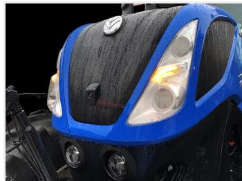
Complete conversion kit for New Holland T-series with LED headlights to replace the cold white LED DRL light. The bright high power LEDs give you plenty of light. They are mounted on an aluminum plate like the original, which ensures optimal cooling and extended lifetime on the LEDs.
