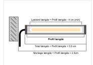
Completely assembled Matronics IP65 Lightbar (Anodiseret) (Anodized) 49cm length, with 12V Warm white 3000K LED strip.
