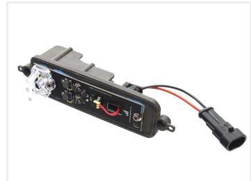
Complete conversion kit for Valtra T, N, and Q-series with LED headlights to replace the cold white LED DRL light. The bright high power LEDs give you plenty of light. They are mounted on an aluminum plate like the original, which ensures optimal cooling and extended lifetime on the LEDs.
