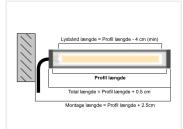
Completely assembled Matronics IP65 Lightbar (Anodiseret) (Anodized) 149cm length, with 12V Warm white 3000K LED strip.
