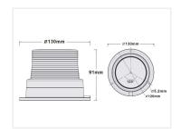
Classic LED beacon light in our Prostrobe series, a durable and waterproof design. The rotor beacon is R65 approved. Clear warning light with  $24 \times 1W$  LEDs and 7 strobe functions:
