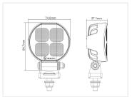
Round E-approved LED lamp with 12 powerful Osram LEDs. Aluminum housing with durable powder coating and stainless steel brackets. The light color is 5700K, and the 90-degree optics provide good and broad light distribution.
