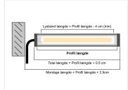
Completely assembled Matronics IP65 Lightbar (Anodiseret hjørne) (Anodized corner) 100cm length, with 12V Neutral white 4000K LED strip.
