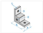
Corner bracket in solid aluminum, with M6 sidehole, which can be used for feet, wheels, or to attach a plate. The bracket is typically mounted at the bottom of a frame, where it is fastened with two M6 bolts.
