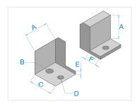
The aluminum bracket is attached at the end of series 30 profiles, where the large M8 hole (drawing B) makes it easy to mount casters / transpor wheels or a foot. Only a single M8 bolt and a T-nut are needed to secure it.
