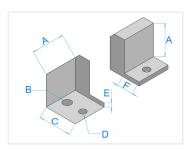
Aluminum end fitting with M6 hole, mounted at the end of a Series 20 profile. Can be used for a foot or transport wheel. Only a M6 bolt and T-nut, or hammer bolt and nut are needed for installation.
