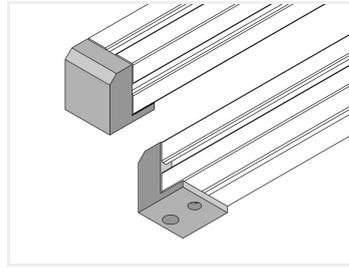
Aluminum bracket that screws into the end of a Series 40 profile. The large block has an M12 thread at the bottom (drawing B), for example, for a foot or for casters / transport wheels. You need an M8 bolt and a track-nut, or a hammer-bolt and a nut to fasten it to a profile.
