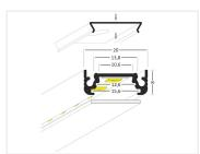
Completely assembled Matronics IP65 Lightbar (Anodiseret) (Anodized) 49cm length, with 12V Neutral white 4000K LED strip.
