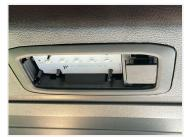
LED light source replacing the original ones in the reading lights in the ceiling of MAN TG 2023+.
