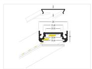
Completely assembled Matronics IP65 Lightbar (Sort) (Black) 200cm length, with 12V Warm white 3200K LED strip.
