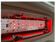
Powerful LED light source that replaces the original light source in the interior ceiling lamps of TGS and TGX +2020.
