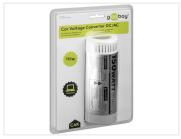
A voltage inverter that converts 12 V DC to 230 V AC, so that you can connect regular 230V appliances to a car, for example. Max power is 150W at 0.65A at 230V. There is also a standard USB plug that can be used for standard USB units. Max. USB current is 2.4A.
