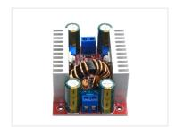
Extra powerful DC step up boost converter that can handle up to peak 400W / 15A input current. The connection is very simple, as there are screw terminals on the input and output, marked "In" and "Out" respectively on the printed circuit board.
