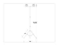
2x30W LED floodlights from Avide on a foldable tripod. The height can be adjusted by using the 2 grips that are placed on the rod. Min. height is 625mm and max. is 1600mm. The legs can be folded for easy transport.
