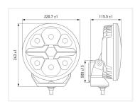
Hella Valuefit Blade 9 inch spotlight high is a new type lamp with a modern design and with integrated LED light and dual color position-light, that is placed in the middle of the lamp. This gives you the possibility to change between white and yellow positions-light as you feel like it so that it fits your vehicle. The yellow position-light is not E-approved.
