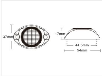
Hideaway type 4 - Bright and compact LED warning strobe lamp, that can be connected to both 12V and 24V, and can be surface mounted on car, MC and truck. The compact oval housing has 4 powerful 3W LEDs, and they create a bright warning together with the special lens, regardless of placement. The LED lamp is made of aluminum, which makes them very robust against harsh weighing conditions.
